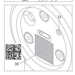
Your SMOOV 010 is ready for use again if pairing was carried out successfully. Remove the QR Code from the drive and operating unit and stick them in the user manual for your safety, so that no unauthorized person can connect another control unit to the SMOOV 010.
